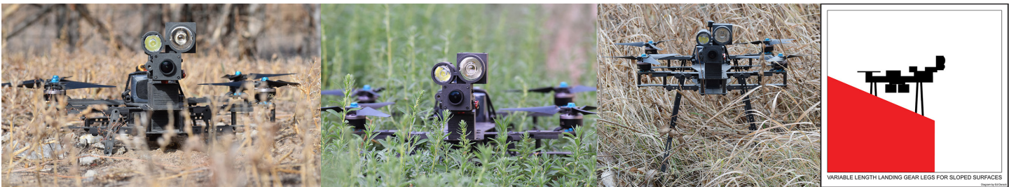
This series of images illustrates the highly versatile landing gear system of the DSA-2. Central to the SUMIDS concept, the landing gear of the DSA-2 can be quickly adapted to a wide variety of surfaces for operation on land. Each landing gear leg is mounted individually with a single bolt and can be adjusted to a wide variety of angles. This allows the DSA-2 to be landed on a variety of terrain for high-endurance ISR and situational awareness building. Shorter landing gear legs may be used for situations requiring the lowest profile for the DSA-2 while operating on land; longer landing gear legs can be used for situations requiring clearance of visual obstacles for the situational awareness module, and landing gear legs of varying length, each leg mounted at an appropriate angle, can be used for sloped surfaces like roofs. CREDIT: Ed Darack
