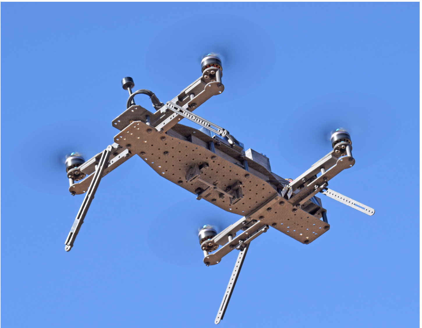
DSA-2 during military flight testing, underside view. View shows easily configurable, open architecture design, easily configurable landing gear system, multiple tie-down points, and 2-hardpoint cargo system. CREDIT: Ed Darack
