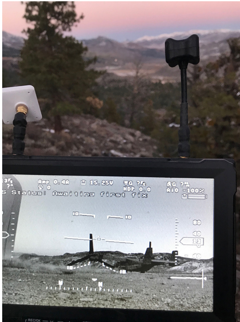
SUMIDS control unit with integrated screen for imagery downlink, showing image of an MV-22B Osprey during exercise at the Marine Corps Mountain Warfare Training Center in which SUMIDS were incorporated to build situational awareness. The operator controlled the situational awareness module from 2.6 miles distant in mountains overlooking the expeditionary airfield, illuminated areas of interest, sparkled notional targets, and marked notional targets with remotely activated marker beacons. CREDIT: Ed Darack
