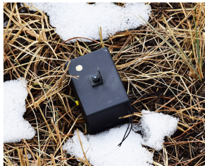
Remotely activated marker beacons that can be carried by the DSA-2 and other Darack Research SUMIDS. Left: detailed view of marker beacon. Middle: Deployed marker beacon. Right: Two side-by-side marker beacons activated at night. Marker beacons may be configured with high-intensity visible wavelength light emitting diodes (LEDs) (of a variety of colors), high-intensity infrared LEDs, or radio frequency emitters. CREDIT: Ed Darack
