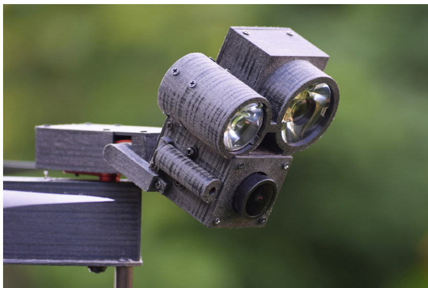
Detailed view of the DSA-2's fully articulating situational awareness module, which comprises a day / night imager, a bore sight mounted laser pointer, a visible wavelength illuminator, and an 850-nanometer infrared illuminator. By mounting the situational awareness module on the upper side of the forward extremity of the DSA-2 ("up and out front"), the system can perform high-endurance ISR and situational awareness building while operating on land due to the configuration's intrinsic high field of view. A user can select an appropriate landing gear configuration, fly the DSA-2 to a predetermined key terrain feature, then pan and tilt the situational awareness module to gather imagery. Operator can then use active systems (laser pointer and illuminators) when needed to build situational awareness for other mission participants. Due to its ability to be powered down remotely, the DSA-2 can have on-station times stretching to days. CREDIT: Ed Darack
