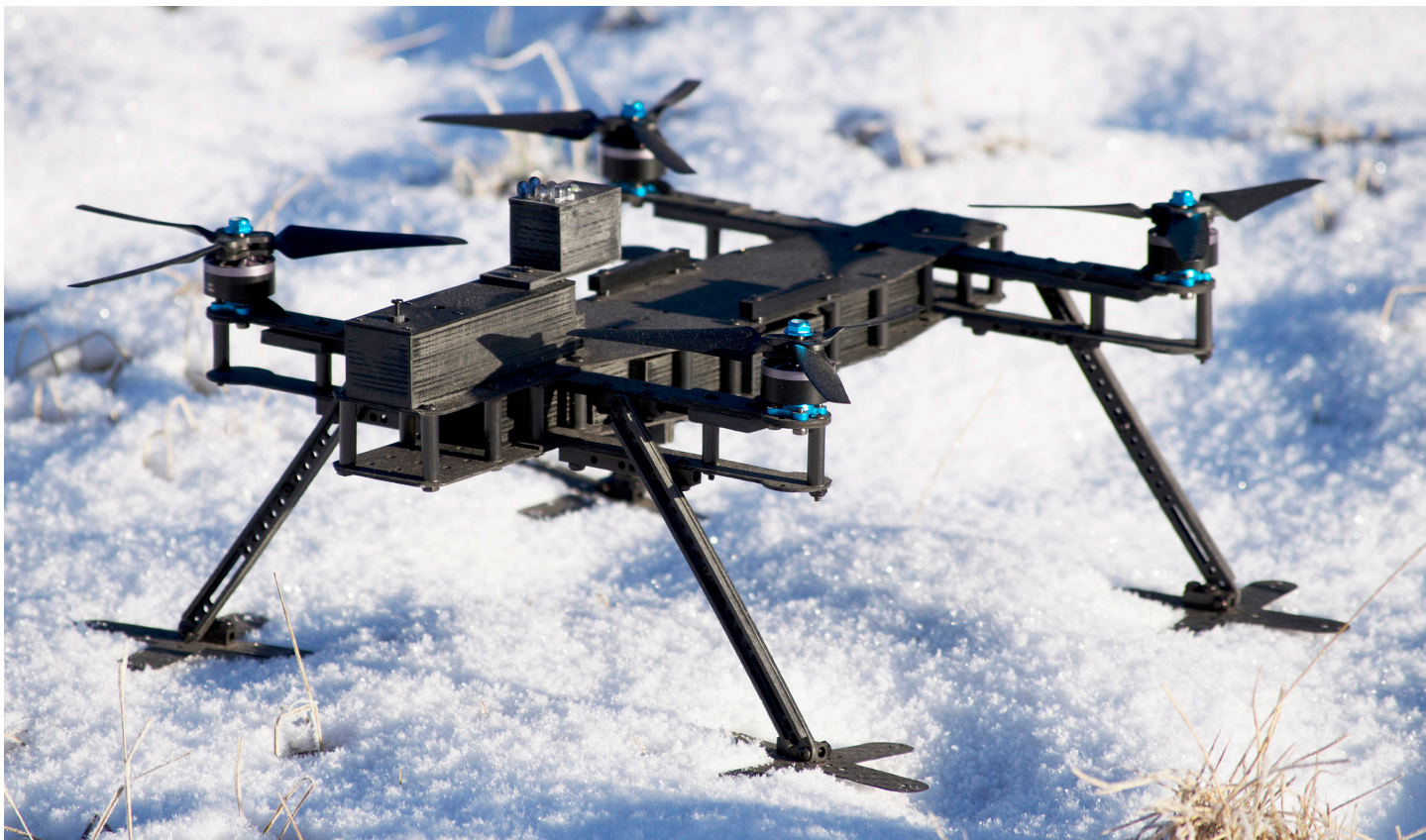
Detailed view of the DSA-2's landing gear system, shown with easily mountable snowshoes attached for snow or mud operations. CREDIT: Ed Darack
