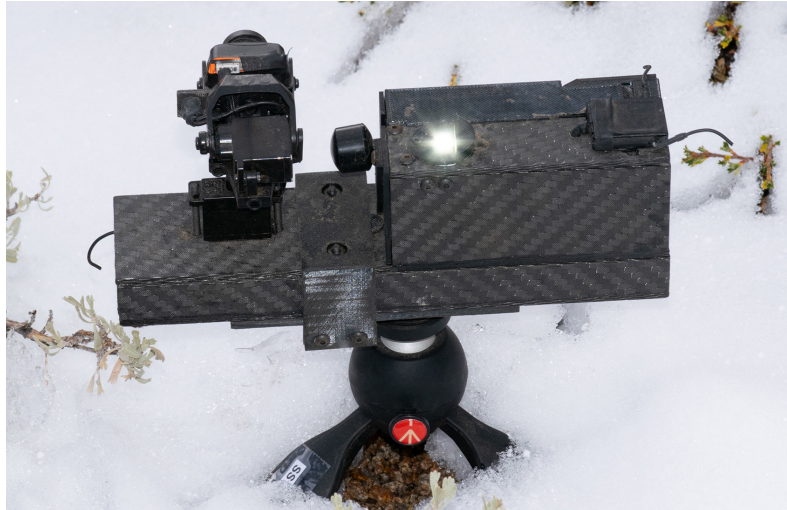
Darack Research Static Surveillance and Targeting Pod (SSTP). The SSTP, which can be carried and deployed by the DSA-1 or DSA-2, is a small pod that comprises a fully articulating day / night imager with a bore sight mounted laser pointer and a self marker. Shown in this image: cold weather testing of the SSTP; self marker activated. CREDIT: Ed Darack
