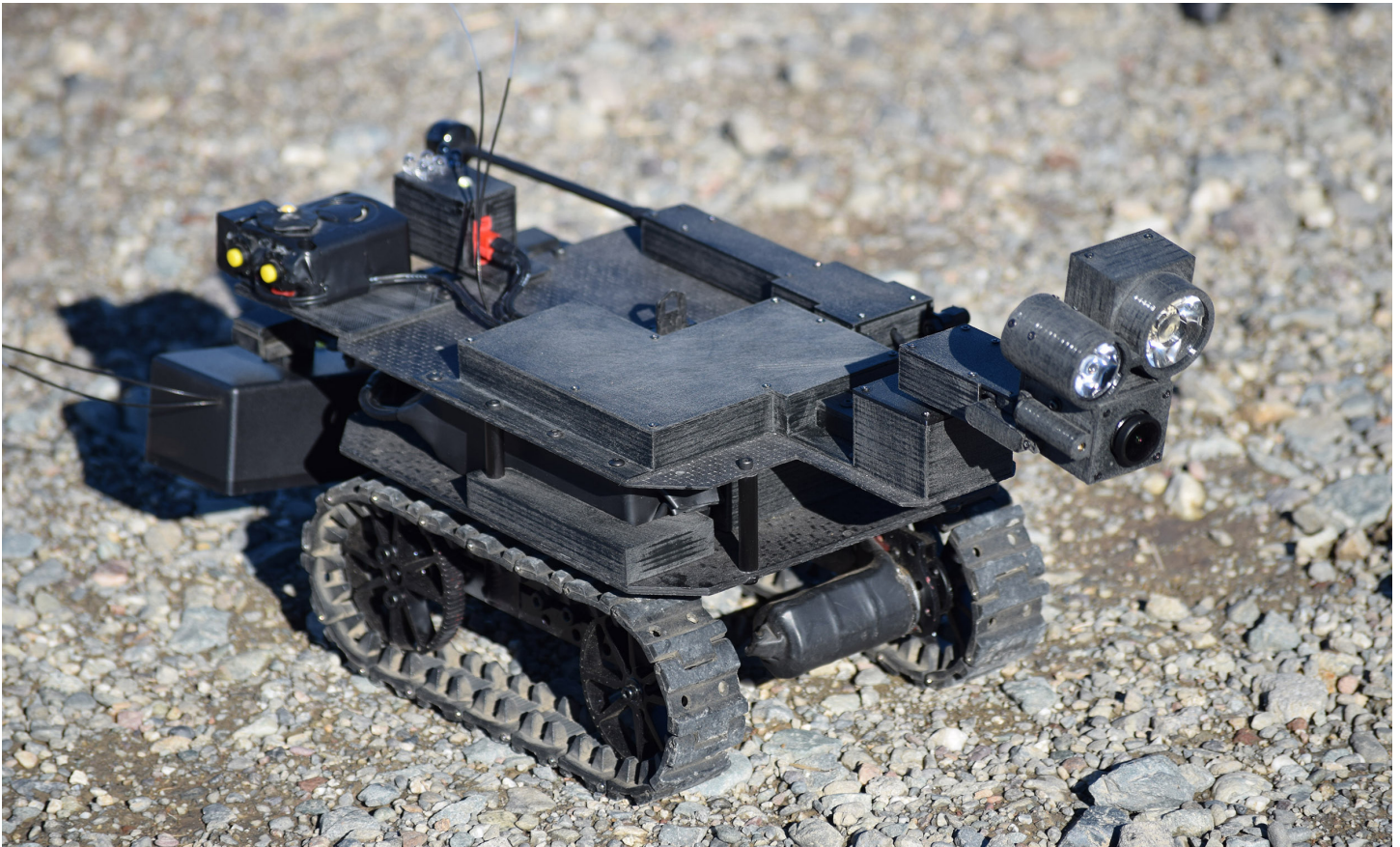
Darack Research Ground Surveillance and Targeting Vehicle (GSTV). The GSTV can be carried by the DSA-1 through the air, deployed on the ground, and then perform ISR and situational awareness building from the ground. It comprises a situational awareness module (day / night imager, bore sight mounted laser pointer, visible wavelength illuminator, and an 850-nanometer infrared illuminator), a 2-point cargo system (to carry marker beacons, as shown in image), and has a form, like the DSA-1 and DSA-2, allowing use for a wide array of applications. CREDIT: Ed Darack
