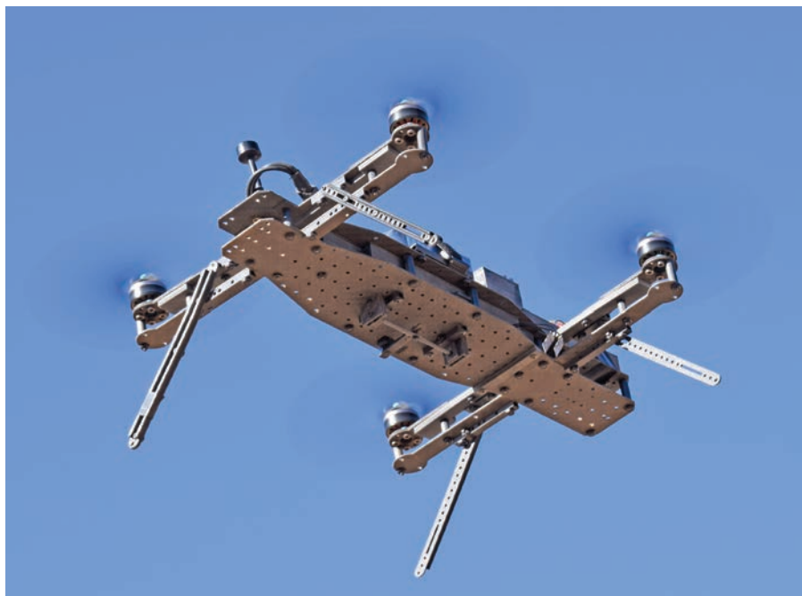
View of a small UAV in flight, showing multiple tie-down points, easily configurable landing gear, and two remotely-actuated attachment points (hardpoints). (Photo by Ed Darack.)
