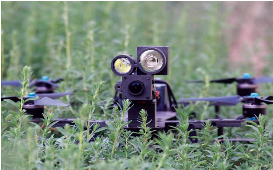
Demonstration of a UAV performing ISR from the ground. The UAV is equipped with an articulating day/night camera, a boresight-mounted laser pointer, a visible illuminator, and an infrared illuminator. This system was designed with its ISR/active situational awareness systems atop the craft for maximum field of view and easily configurable landing gear. Before system deployment, a user would identify key terrain features, determine the length and configuration of landing gear legs based on vegetation, snow depth, etc., fly the system to a key terrain feature, and then could perform ISR with the articulating camera. The user could then sparkle a target, illuminate an area, or deploy remotely-activated marker beacons for landing-zone creation or target marking. (Photo by Ed Darack.)
