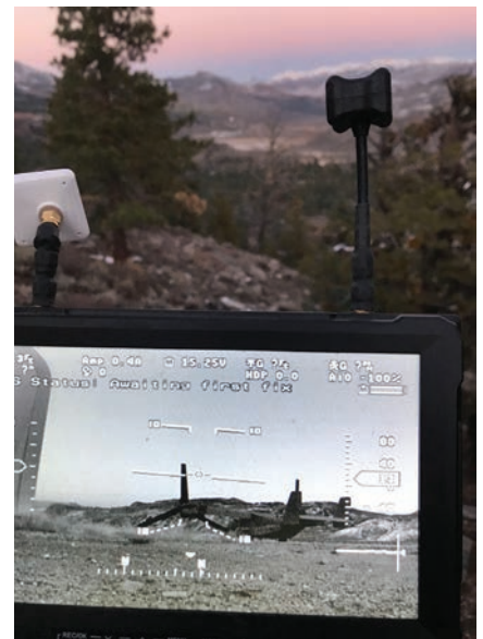
View of a monitor on a C2 unit showing real-time feed from an experimental small unmanned system targeting a Marine Corps MV-22 B Osprey parked at the airfield of the Marine Corps Mountain Warfare Training Center. The user controlled the vehicle from 2.65 miles distant. (Photo by Ed Darack.)
