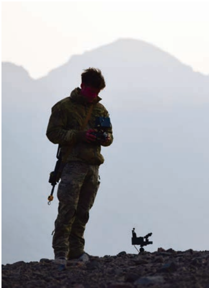
A Royal Marine operates a small surveillance and targeting pod during a training exercise at the Marine Corps Mountain Warfare Training Center. The system comprises a day/night video camera, a self-marker, and a laser pointer boresight mounted to the camera. The system, which can be deployed by a small UAV, can provide persistent ISR and can actively build situational awareness under the command of a remote operator. (Photo by Ed Darack.)
